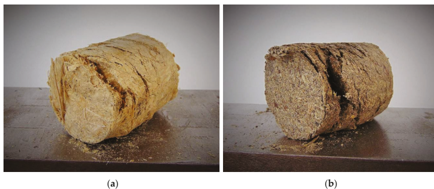
Figure 13. Bio-briquette fuel samples after rupture force testing: (a) bamboo fiber; (b) sugarcane skin.
