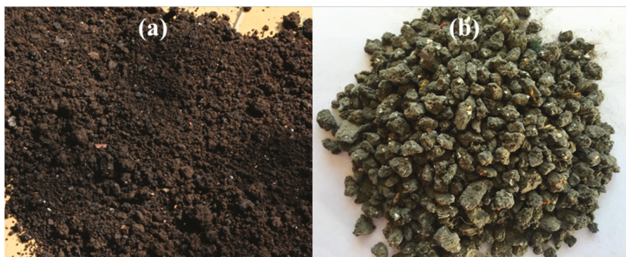
Figure 1. Photograph of sewage sludge, (a) sludge from the wastewater treatment plant and (b) sludge after preheating.
