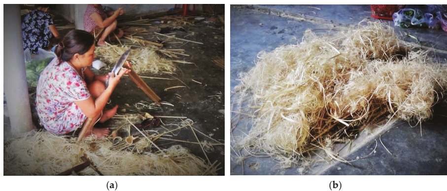
Figure 2. Bamboo processing in Thừa Thiên Huế province, central Vietnam: (a) manual removing of fiber; (b) produced waste biomass: bamboo fibers.
