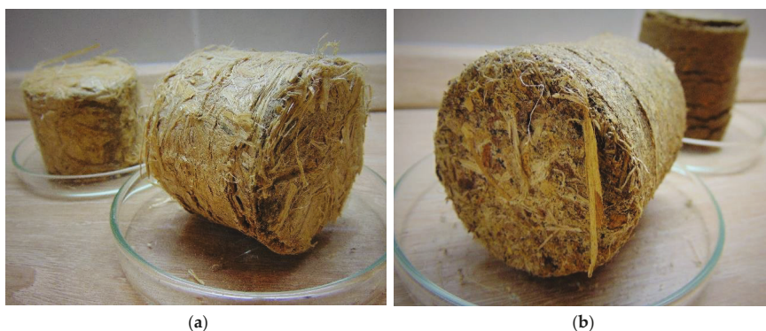
Figure 12. Bio-briquette fuel samples after mechanical durability testing: (a) bamboo fiber; (b) sugarcane skin.
