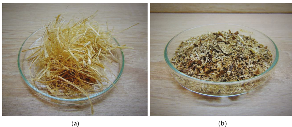
Figure 5. The form of samples prepared for chemical and mechanical analysis: (a) bamboo fiber; (b) sugarcane skin.
