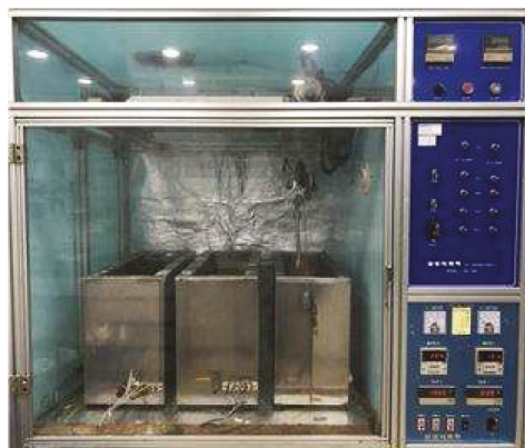
Figure A1. Small batch reactor setup for organosolv only pretreatment.
