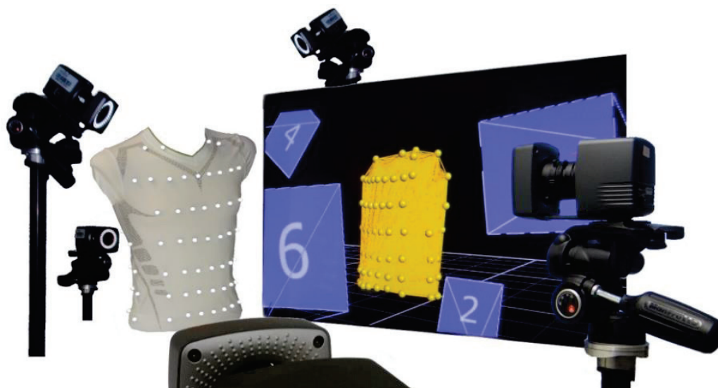
Figure 1. Schematic of the MoCap system. Five of the nine infrared cameras, the compression shirt with MoCap markers and the representation of the MoCap markers by the Vicon Systems on a screen. Figure published in [3].
