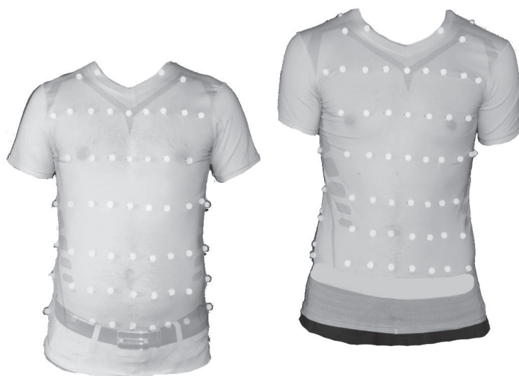
Figure 12. Illustration of variations in anatomical marker positions for subjects of different body shapes (visualized via subject 3 (left) and subject 1 (right)).
