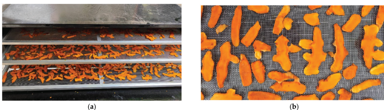
Figure 3. The drying chamber and trays. (a) Drying samples on the dryer tray, (b) Turmeric slices as samples.
