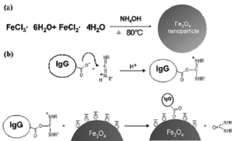
Figure 1. Synthetic route for immobilizing immunoglobulin (IgG) onto the surfaces of Fe 3 O 4 magnetic nanoparticles. Reprinted with permission from [66]. Copyright (2014) American Chemical Society.
