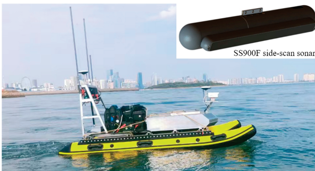
Figure 1. Unmanned surface vessel and SS900F SSS equipment.
