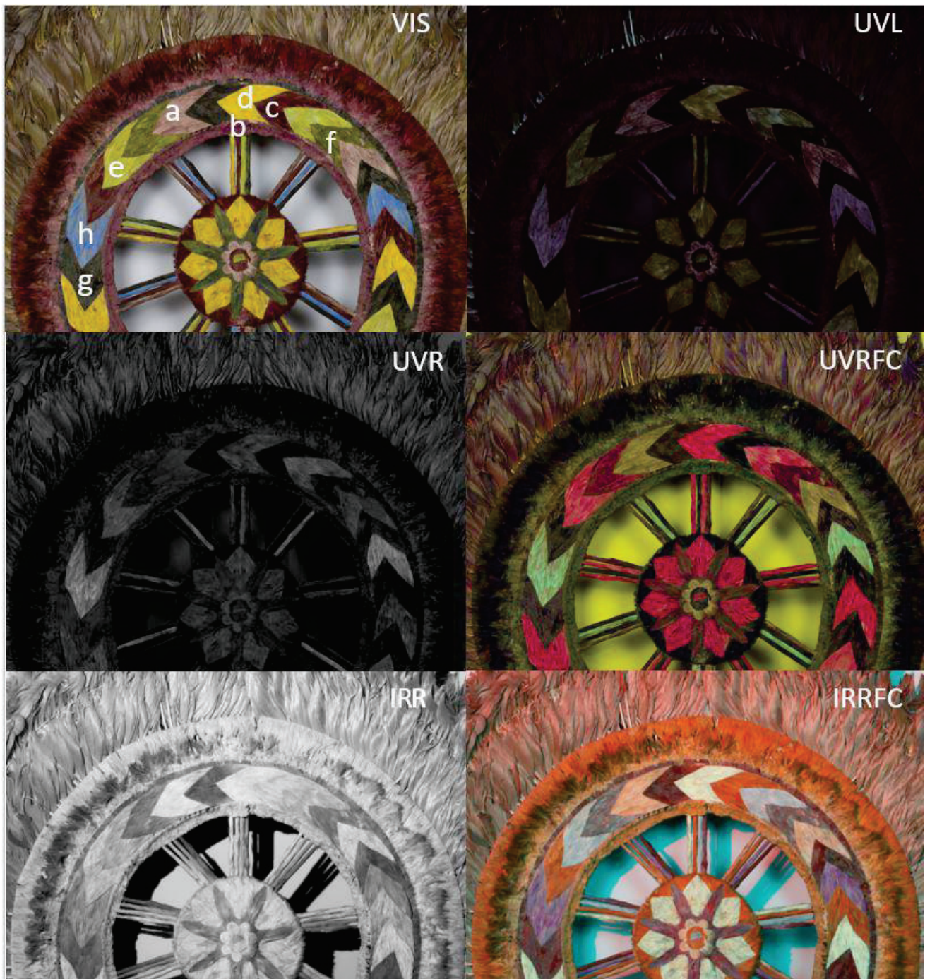
Figure 4. Multiband images (MBI) and false colour images: Set-up by Weltmuseum Wien (see details in Figure 5).
