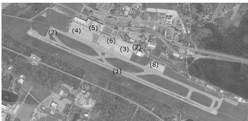
Figure 5. Hypothetical airport layout illustrating the main operational areas of airport infrastructure, numbered (1)–(8) according to the descriptions in Table 1.
