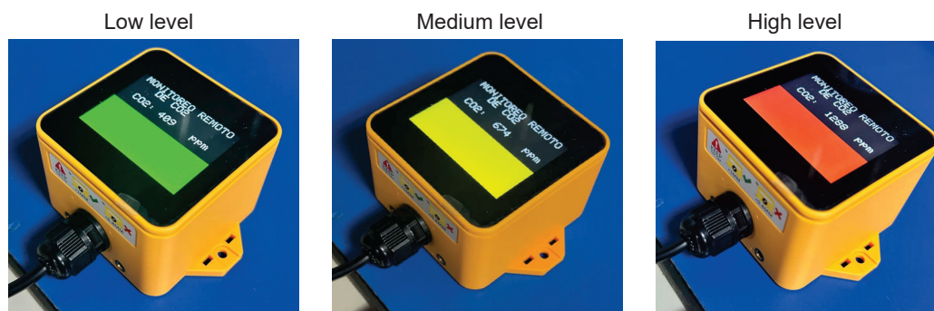
Figure 4. CO 2 concentration levels with indicator colors.
