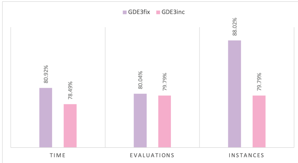
Figure 3. Resource consumption reduction achieved by the proposals GDE3fix and GDE3inc. The plot presents the average reductions concerning the GDE3 procedure in terms of computational time, the number of evaluations, and the number of instances used when evaluating the individuals.
