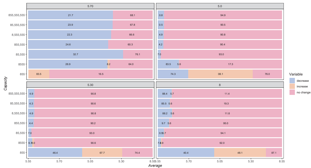
Figure 4. Proportion of generations in which the number of repeated fitness individuals increased, decreased, or remained unchanged during the execution of the GGA-CGT with random gene sorting.
