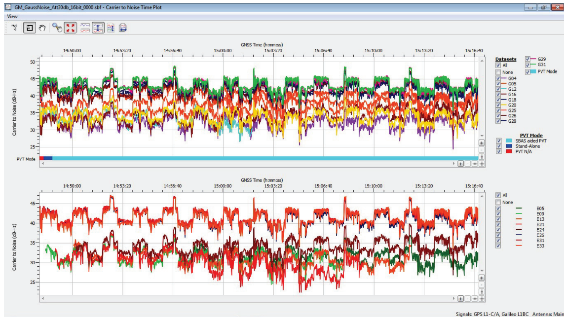
Figure 5. C/N_0 for the satellite considered in this study with the impact of the Gaussian noise (moderate level: 30 dB attenuation) for the 16 bit playback.
