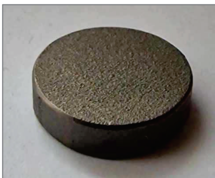
Figure 1. Ti6Al4V ELI titanium alloy substrate prepared using the SLS method.
