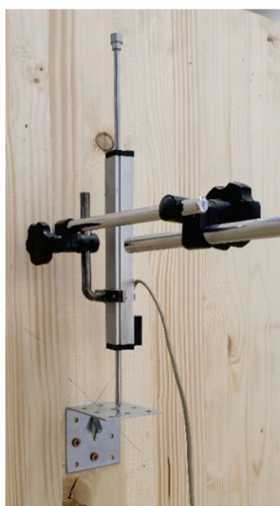
Figure 4. Displacement tracer—sensor from company Ahlborn [42].
