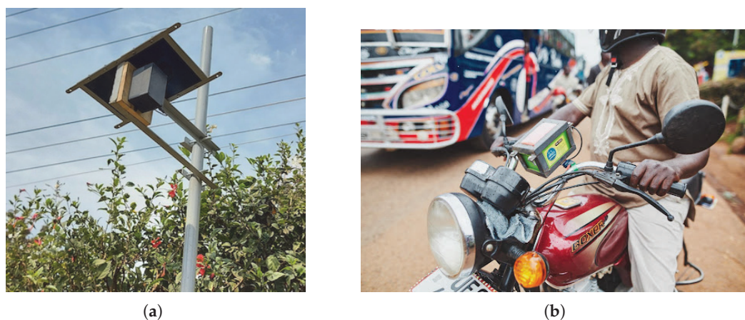
Figure 3. Flexible deployment options for high resolution air quality sensing. (a) Static pole deployment. (b) Mobile deployment.
