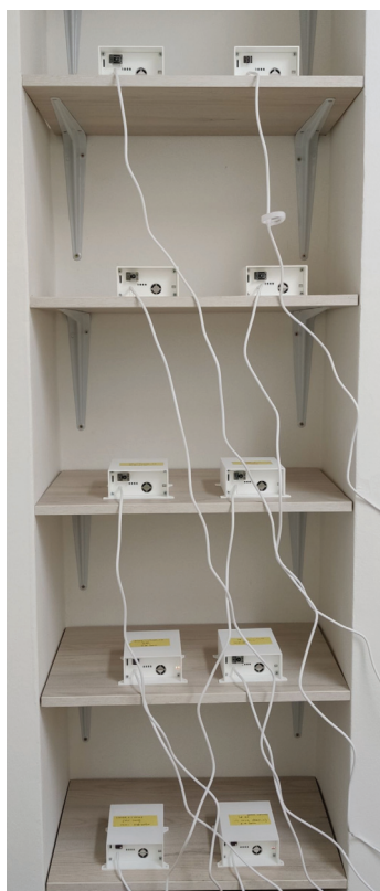
Figure 4. Calibration of MAQS sensors: batch of 10 sensors that are being calibrated in our laboratory for particulate matter spectroscopy and gravimetry.
