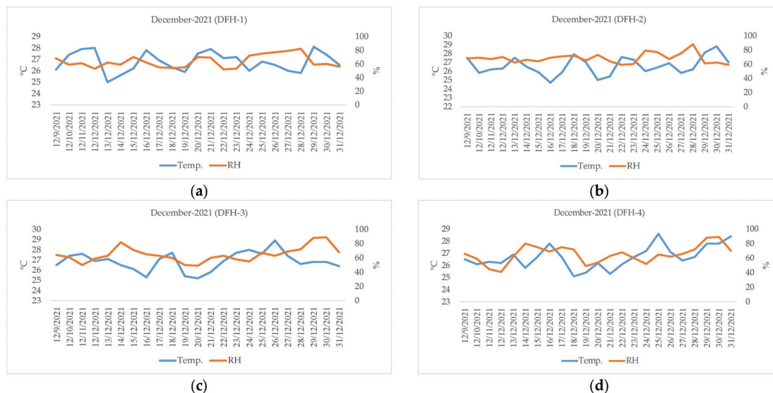
Figure 12. Air temperature (°C) and RH (%) measured from LCSs during the period from 9 to 31 December 2021: (a) DFH-1, (b) DFH-2, (c) DFH-3, and (d) DFH-4.
