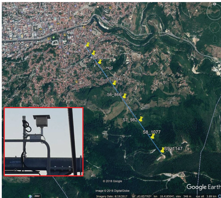
Figure 14. Sarajevo cable car pillars (yellow markers) and terrain from Google Earth. A MAQS sensor is shown in red box.
