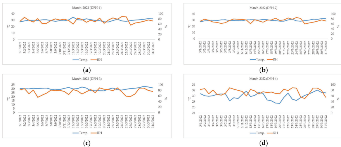
Figure 15. Air temperature (°C) and RH (%) measured from LCSs during the period from 1 to 31 March 2022: (a) DFH-1, (b) DFH-2, (c) DFH-3, and (d) DFH-4.
