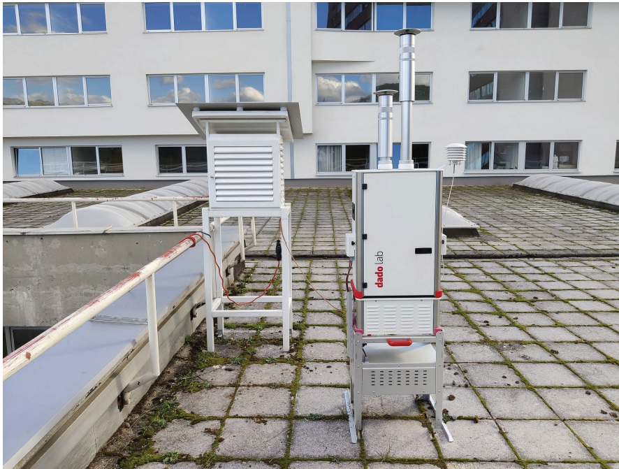
Figure 5. Dual air sampler and Stevenson screen with MAQS sensors inside.
