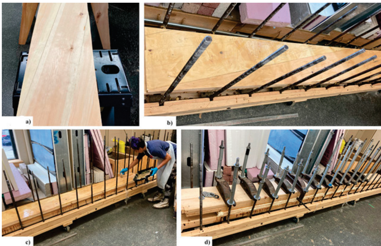
Figure 5. From top left, (a) cutting of boards to desired grain orientation (representative sample at 10^\circ ), (b,c) DCLT panel's gluing process, and (d) DCLT panel's pressing process.
