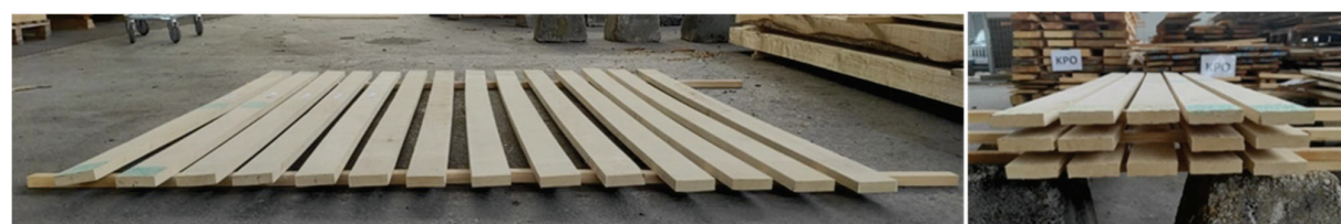
Figure 12. Lumber without spiral grain after the three-month research.
