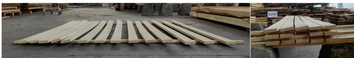
Figure 11. Lumber with spiral grain after the three-month research.
