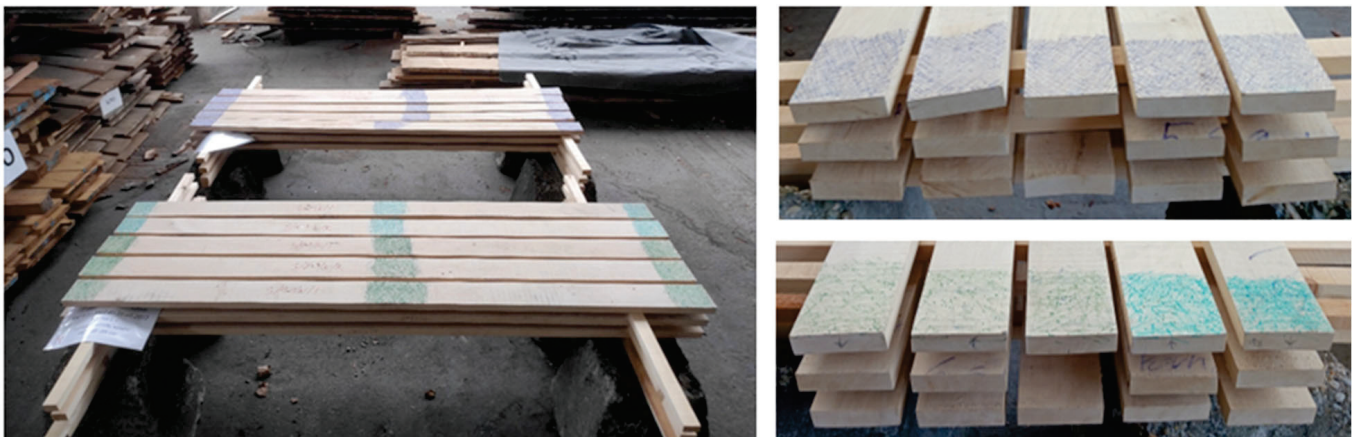
Figure 4. Drying stack for lumber with (pattern of blue) and without (pattern of green) spiral grain.
