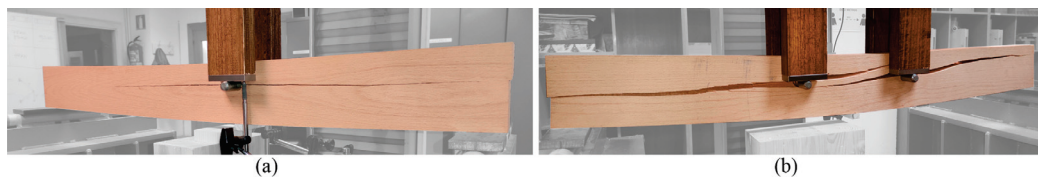
Figure 8. Typical failures: (a) straight and continuous crack; (b) oblique and discontinuous crack.
