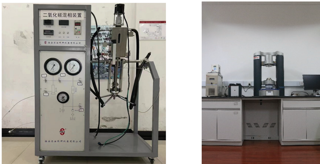
Figure 3. CO 2 fracturing fluid preparation and rheological testing device.
