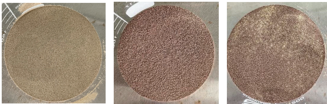
Figure 3. Images show 70/140 mesh ceramic beads (left), 40/70 mesh ceramic beads (center) and 3:2 mixture (right).
