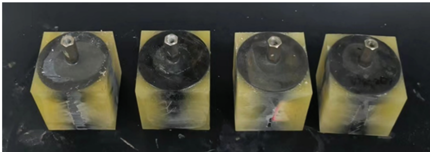
Figure 2. Cemented core with stainless steel wellbore.
