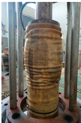
Figure 12. Failure mode of the gravel-over-sand layered sample under 400 kPa confining pressure.
