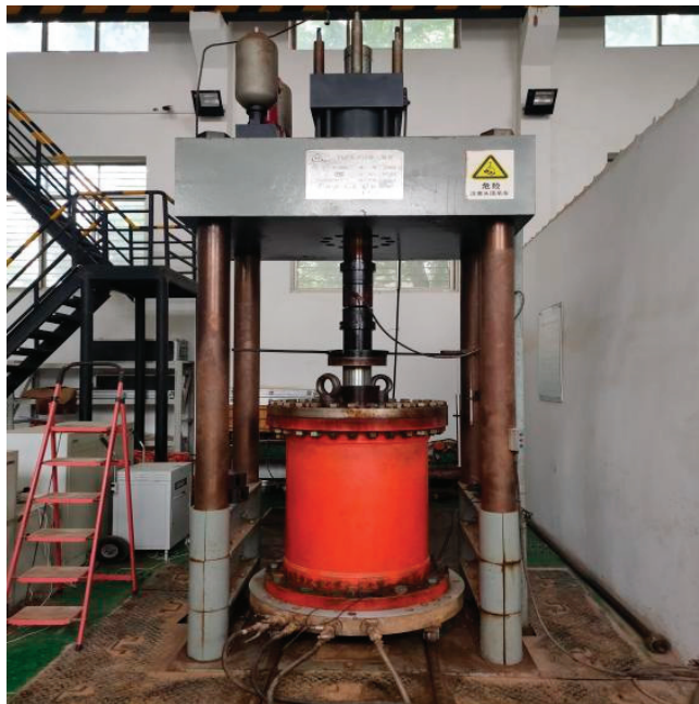
Figure 6. Large-scale triaxial test apparatus.
