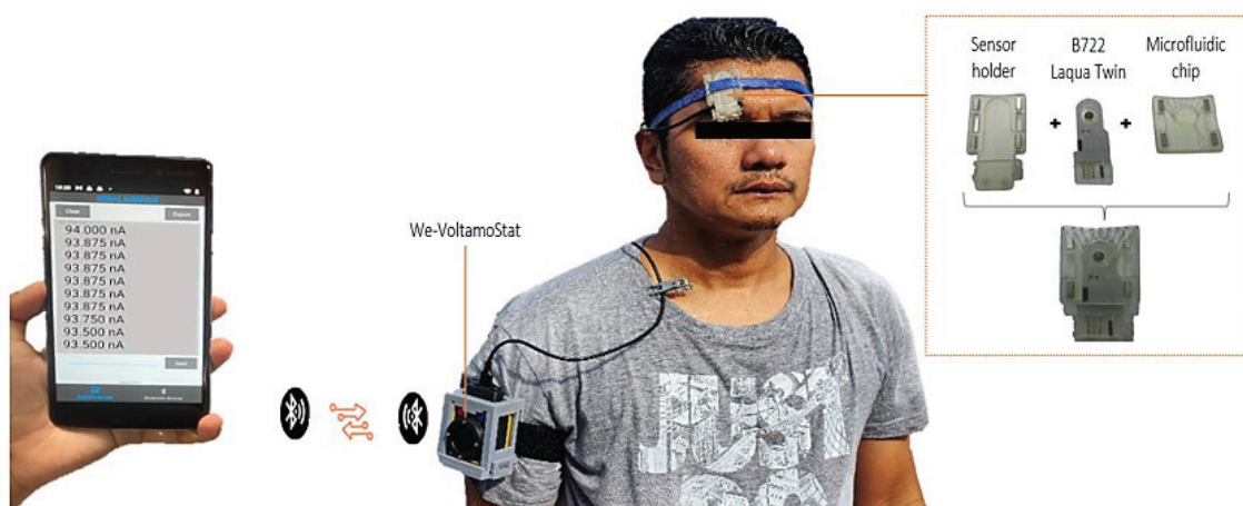
Figure 5. Wearable microfluidic sweat-sensing system during real-time monitoring. The microfluidic chip is worn on the forehead, with data transmitted wirelessly to a smartphone app for continuous sodium analysis.
