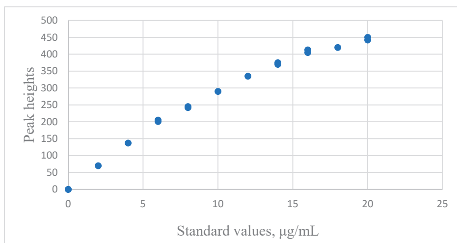
Figure 4. The distribution of the albumin concentration data for the peak heights versus the standard concentrations with spectrophotometry.
