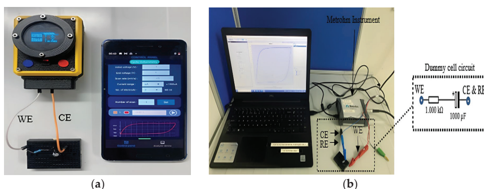
Figure 4. Dummy cell test configurations for validating the We-VoltamoStat. (a) Simplified two-electrode setup with the We-VoltamoStat, demonstrating its reliability in measuring electrochemical currents. (b) Standard three-electrode setup using the Metrohm instrument.
