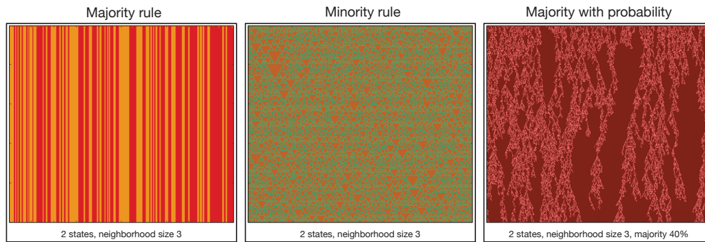
Figure 1. Examples of cellular automata with two states and a neighborhood size of 3, applying majority, minority, and majority with probability evolution rules.
