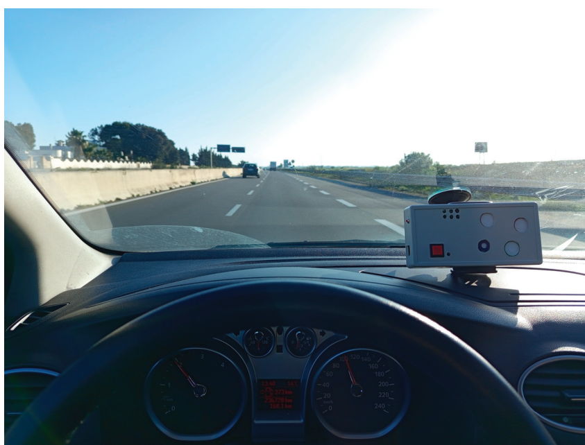
Figure 6. The monitor used for mobile measurements arranged on the car dashboard by using a standard smartphone holder.
