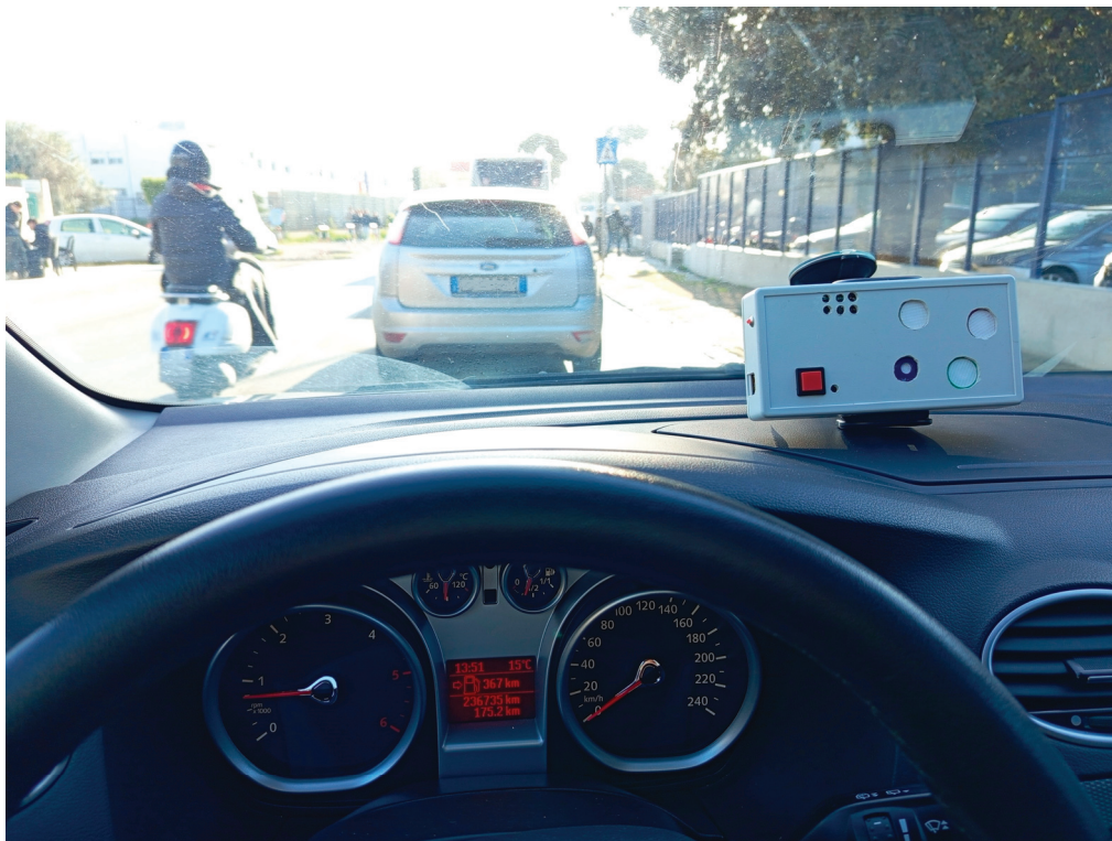
Figure 15. This figure shows the car stopping in a queue caused by heavy traffic, in which a remarkable peak of CO and \text{NO}_2 concentrations was registered by the monitor arranged on the car dashboard.
