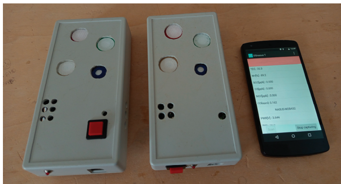
Figure 1. On the left of the figure we can find two monitors, DSnasus, implemented in our laboratory, while on the right there is the smartphone device used for the experiments showing the App running. The sizes of the DSnasus monitors are 17 cm × 8.5 cm.
