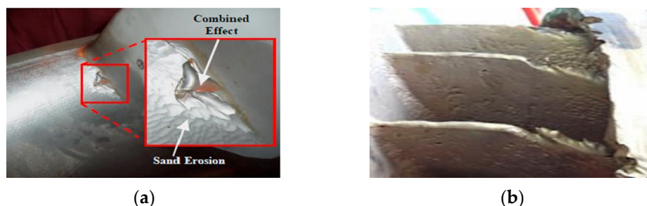
Figure 1. Erosion in the hydro turbines. (a) Turbine runner with synergy of cavitation and sediment erosion, (b) synergistic damage caused by particles and cavitation at the leading edge of the runner blades.
