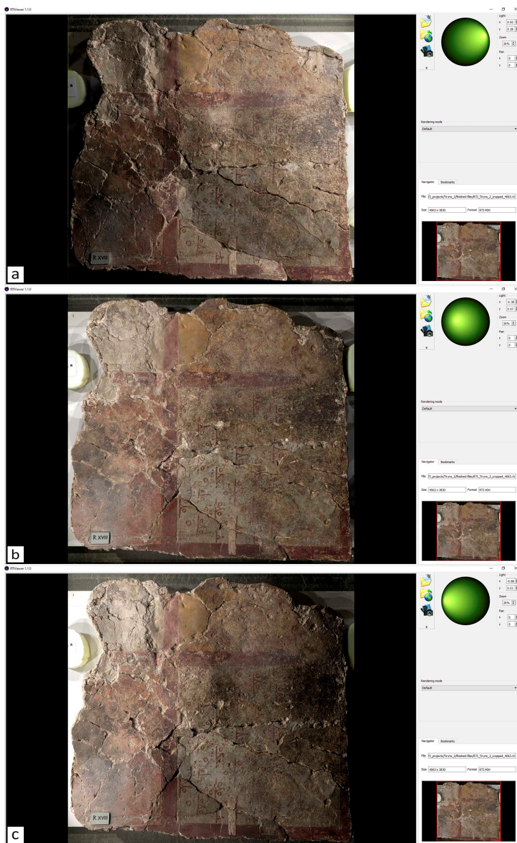
Figure 17. (a–c) Screenshots from RTIViewer demonstrating the adjustment of the green sphere (top right) to simulate varying light directions for enhanced surface analysis.
