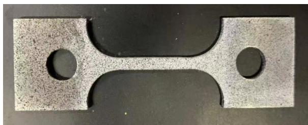
Figure 2. The plate tensile specimen following speckle spray treatment.
