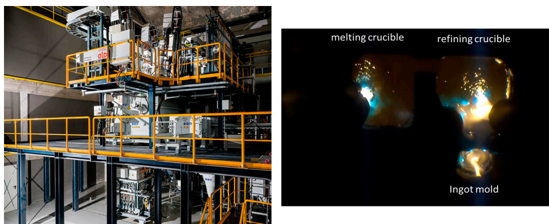
Figure 2. IRT-M2P' pilot furnace (left) and top view of the crucibles during processing (right).
