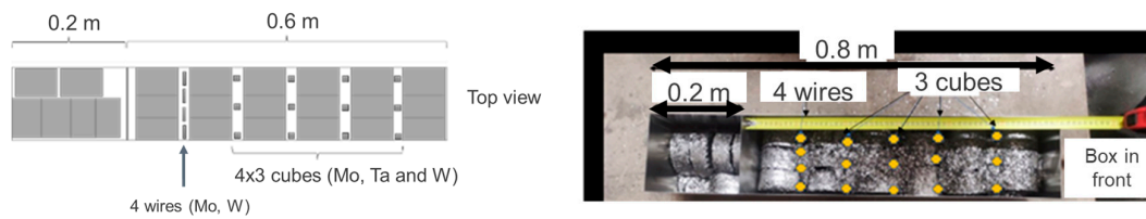
Figure 4. Arrangement of the HDIs in the Ti64 briquette box ( left ), and photograph of the box after deposition of the first briquette layer ( right ).
