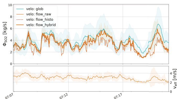
Figure 11. Emission rate retrieval. Emission rates (top) and plume velocities (bottom) of the Etna example dataset on 16 September 2015 between 7:06 a.m. and 7:22 a.m. UTC using the retrieval line “PCS” shown in Figure 8. The analysis was performed using (1) a global velocity of 3.5 m/s (cyan, from cross-correlation analysis); (2) the raw output of the Farneback algorithm (thin orange); (3) using the flow_histo method (thin dashed brown) and (4) using the flow_hybrid method (bold orange). The retrieved effective velocities are plotted in the lower panel and correspond to the average velocities along the PCS line using the flow_hybrid method. Uncertainties are displayed as shaded areas.
