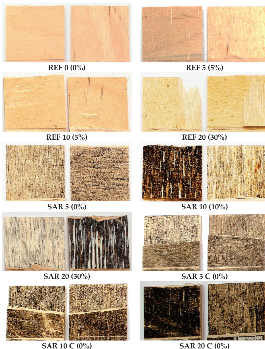
Figure 4. The images of the break zones of the samples after the shear strength test (dimensions: 25 \times 25 \text{ mm}^2 ; numbers in brackets are the estimation of in-wood damage).
