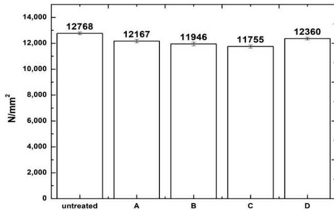
Figure 4. MOE of untreated and PF resin-treated beech wood samples. (A) M_w values of 237 g/mol, (B) M_w values of 305 g/mol, (C) M_w values of 403 g/mol, (D) M_w values of 520 g/mol.
