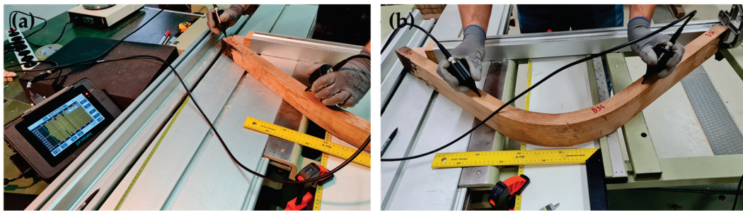
Figure 5. Determination of the velocity of ultrasound (Proceq PL-200PE) in the straight part ( v_S ) (a) and in the bent region ( v_B ) of solid oak specimens (b).
