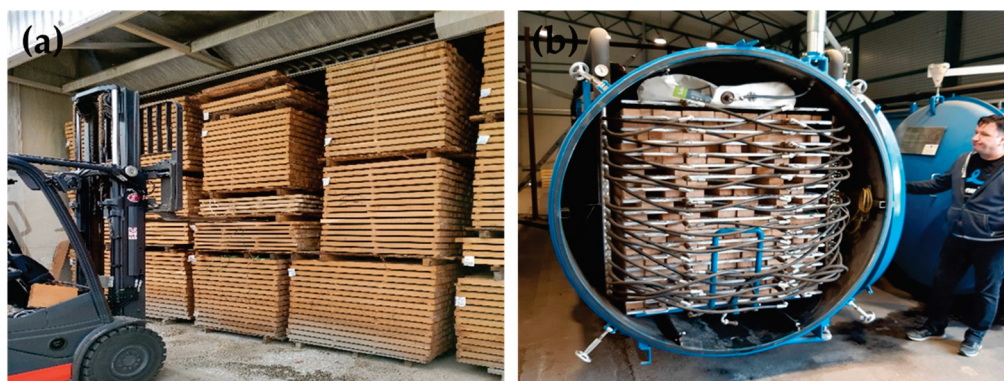
Figure 2. Normal temperature convection kiln drying (KD) of test oak samples (a) and vacuum drying (VD), using hot plate method for heat transfer (b).
