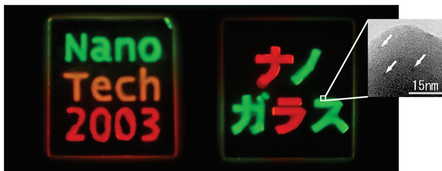
Figure 4. Fluorescent color images of the prepared bulk-type glass containing QDs under UV lamp excitation at 365 nm. The phosphor is selectively adhered to patterned grooves on the surface of the glass substrates, enhancing localized emission [55]. The non-English term (nano glass in Japanese) is the name of research project sponsored by a funding agency (NEDO). The color variation is due to the different size of aqueous CdTe-based QDs.
