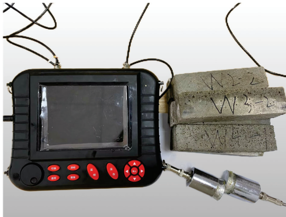
Figure 7. Ultrasonic tester for self-repairing cement mortar specimens.
