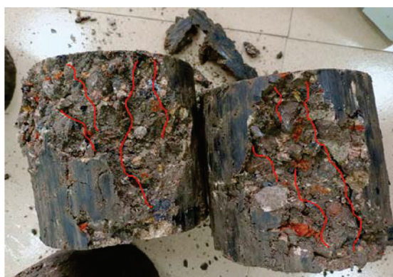
Figure 7. Crushing of representative test pieces (on the left is the A1 group test piece, and on the right is the B1 group test piece).
