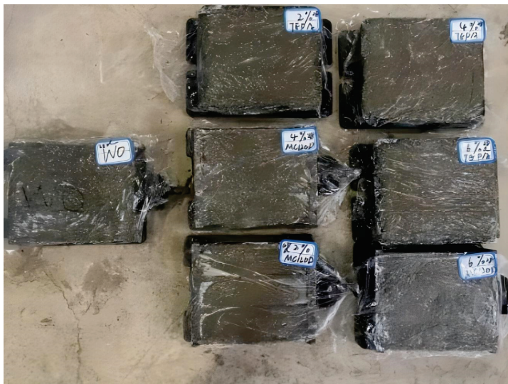
Figure 4. Self-healing mortar repair performance and effect of specimens during indoor film curing.
