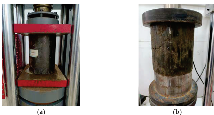
Figure 2. Representative photos of test: (a) specimen compaction; (b) unconfined compressive strength test.
