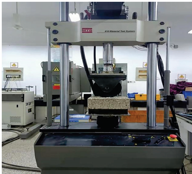
Figure 10. Fatigue Strain Test Data Acquisition System.
