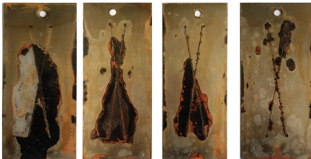
Figure 6. Photographs of the coatings taken after 650 and 720 h of exposure to a 3.5% NaCl solution.
