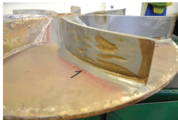
Test rotor blade with WC Co Cr coating (HVOF) HV_{0.2} = 1369
