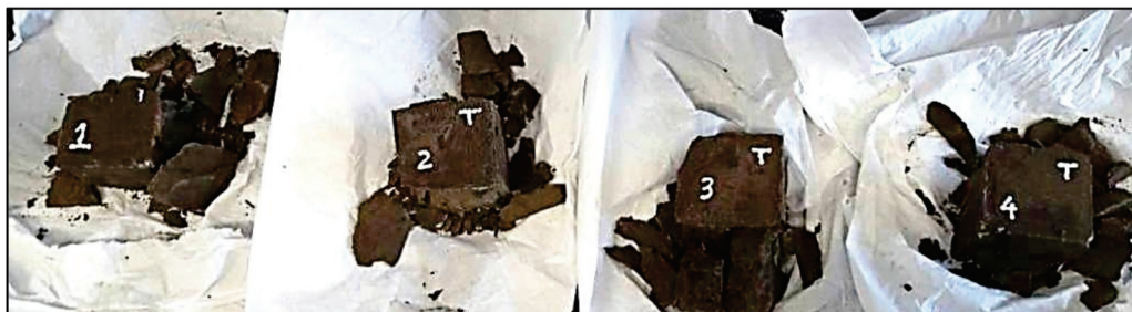
Figure 19. Failure mode of the samples subjected to compressive-strength tests.
