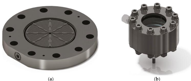
**Figure 2.** CAD schematic of the radial flow reactor: (a) The microstructure in detail including the space between the pins, which is filled with catalyst particles. The reactants are entering in the center and the reaction mixture flows from the inside to the outside and is removed in the form of a ring. (b) View of the reactor. A look inside is possible by using a glass plate pressed onto the structure.
