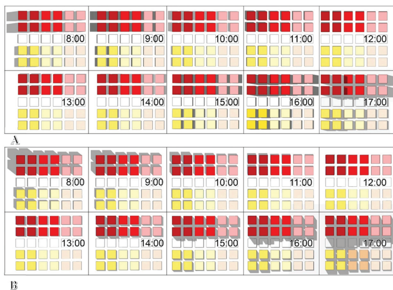
Figure 5. Shading distribution for each AR per hour from morning to sunset: (A) north orientation; (B) northeast orientation. Created using SketchUp after aligning the model to the original location of Cairo city.
