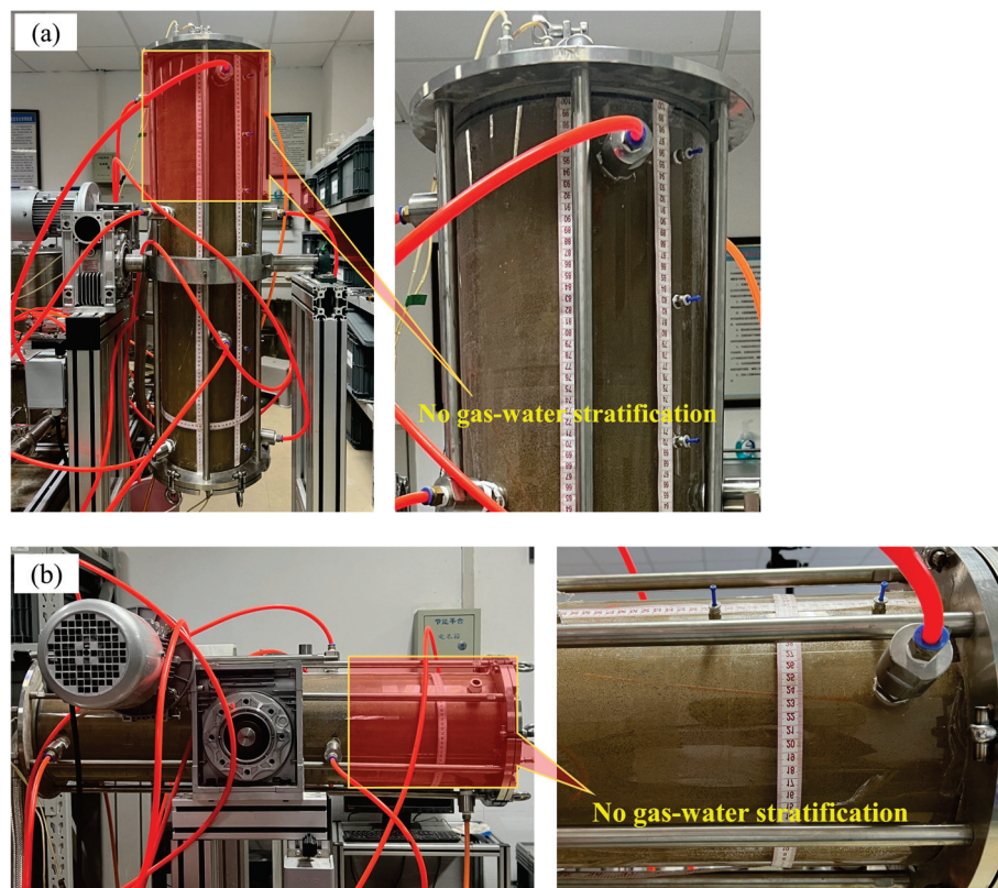
Figure 20. The uniform inflow of gas–water in vertical and horizontal wells with GP completion: (a) vertical well with GP completion; (b) horizontal well with GP completion.
