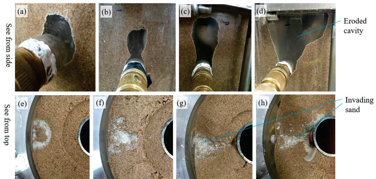
Figure 4. Observed erosion and sand invasion patterns in packed quartz sand with different compaction degrees. (a,e) Compaction degree of 100%. (b,f) Compaction degree of 98%. (c,g) Compaction degree of 96%. (d,h) Compaction degree of 95%.
