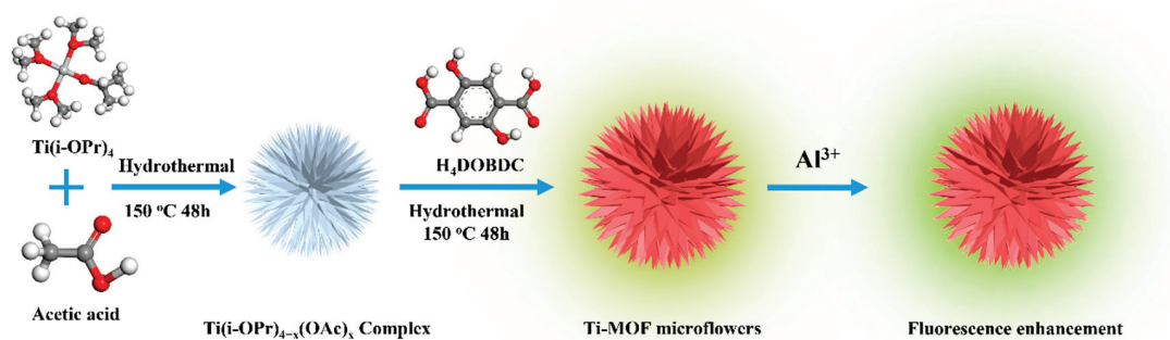
Scheme 1. Schematic illustration for manufacturing hierarchical Ti-MOF microflowers and Al(III) ions luminous sensing.
