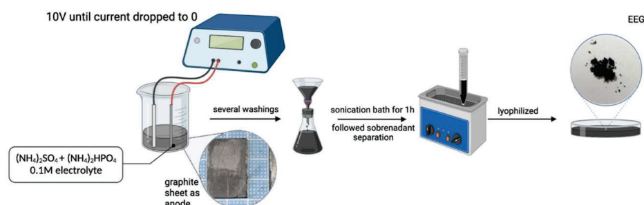
Figure 2. Electrochemical exfoliation method (reprinted from [32], with permission from Elsevier, license number: 5595791108264).
