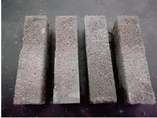
Figure 10. The macroscopic morphology of the specimens after the freeze–thaw cycle test.
