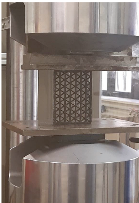
Figure 4. Buckling test of the 30% isogrid.
