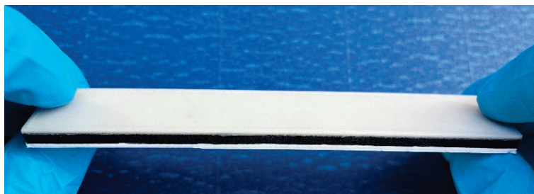
Figure 4. Example of the printed sandwich specimen (volume fraction ratio 1:2:1, material stacking order: PLA/ePLA-LW/ePLA-GF).
