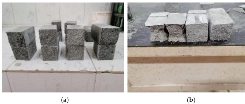
Figure 4. The macroscopic morphology of the specimens. (a) The macroscopic morphology of the specimens after the flexural strength test. (b) The macroscopic morphology of the specimens after the compressive strength test.
