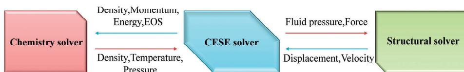
**Figure 1.** Coupling mechanism between the chemical solver of CESE and structure.
