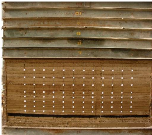
Figure 7. Diagram of the displacement measurement points.
