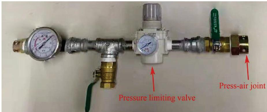
**Figure 4.** Installation position of pressure limiting valve.
