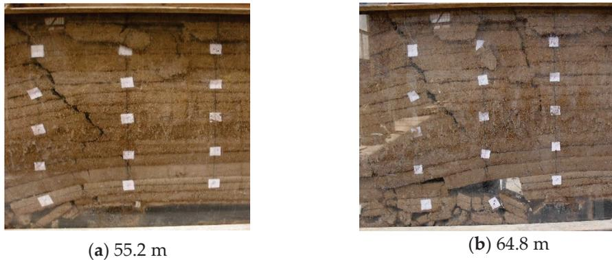
**Figure 10.** The crack in the working face during coal mining.
