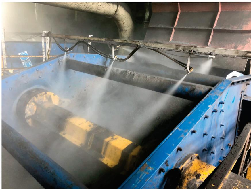
Figure 1. View of the PASAT sprinkler system.
