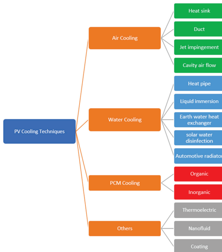
Figure 3. Classification of cooling techniques.
