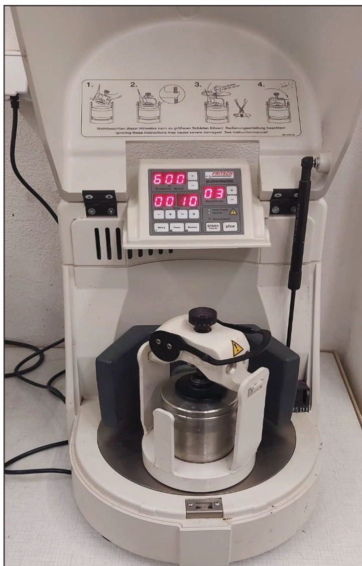
Figure 7. The appearance of the ball mill (Pulverisette 6) used for micronization.
