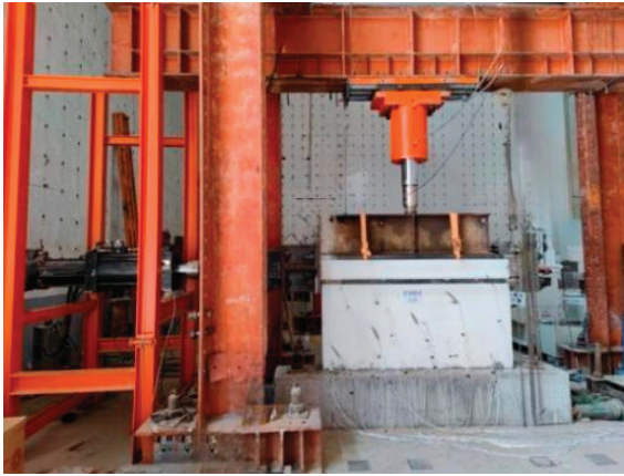
Figure 4. Test loading device.
