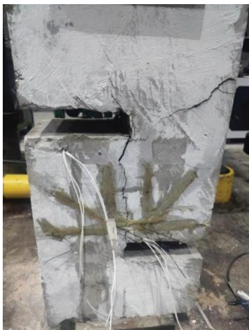
Figure 6. The failure mode of sample ZJ2 (front).
