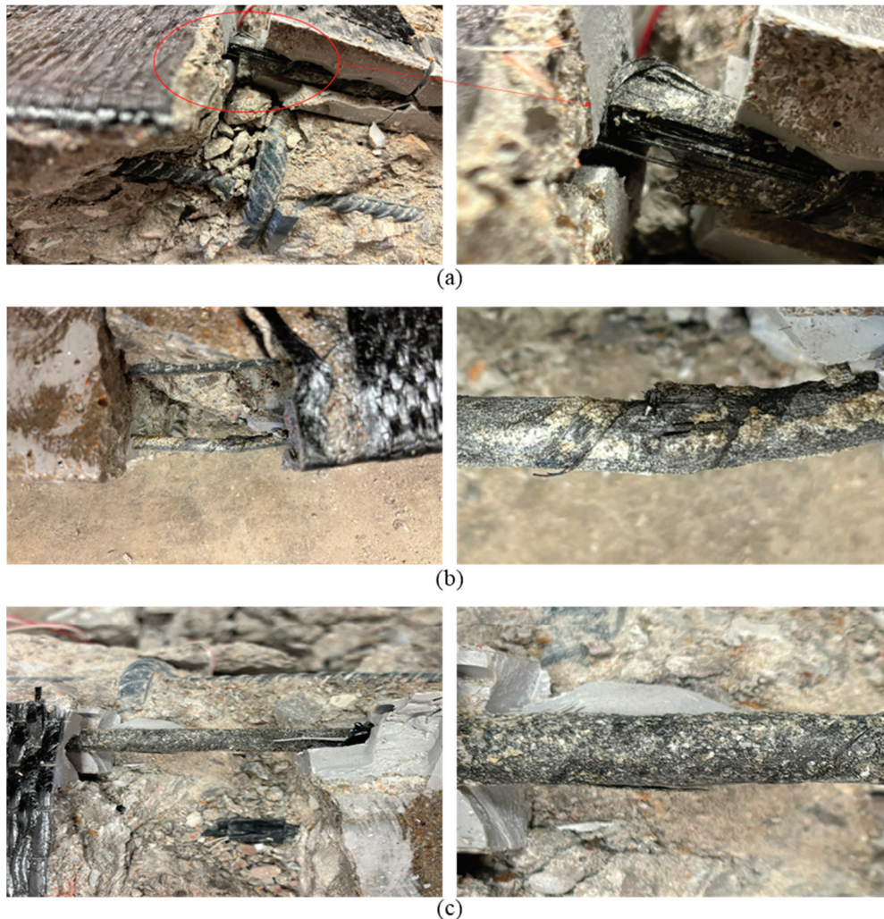
Figure 16. Various failure modes of RC beams strengthened with NSM-CFRP, (a) type NU beams, failed by the CFRP bar rupture, (b) type NSU beams, failed by the CFRP bar rupture, (c) type NSU beams, failed by sudden spilling of the epoxy cover.
