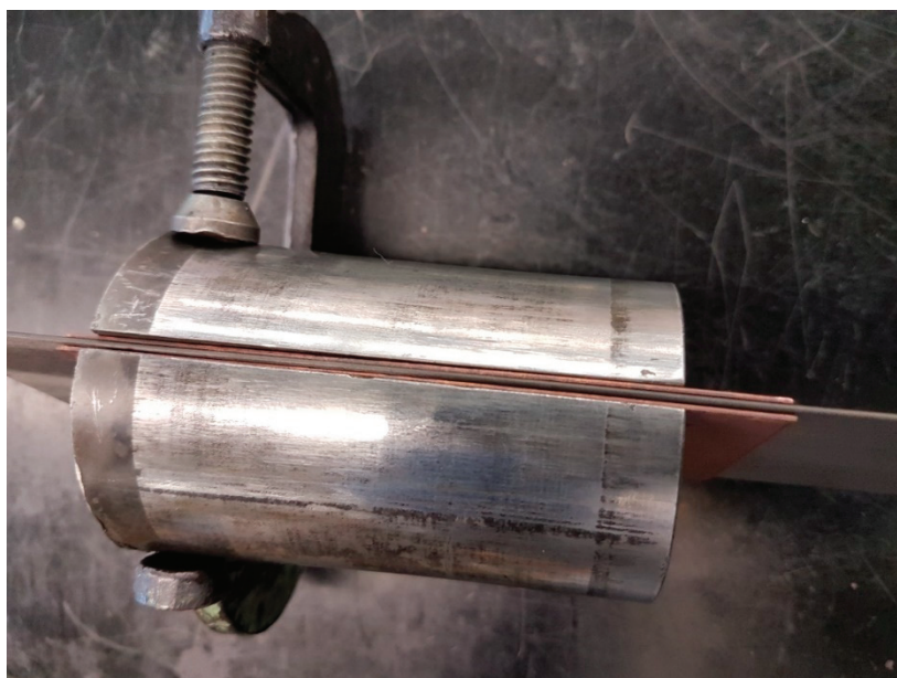
Figure 2. Assembled CFRP plate, sleeves, and wedges before lubrication.
