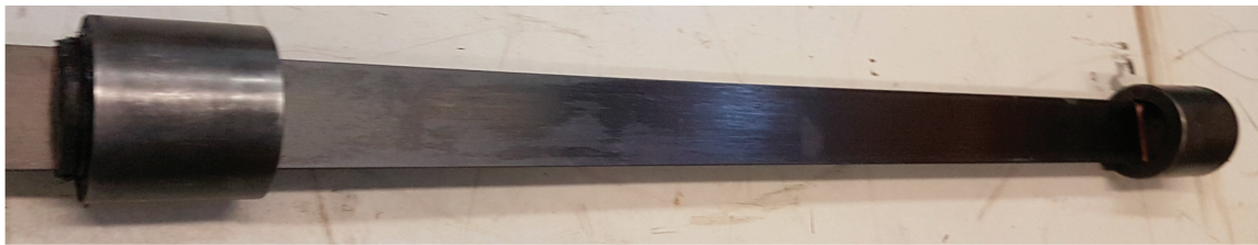
Figure 3. Assembled wedge anchorage (left), dead-end anchorage (right), and CFRP plate.
