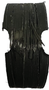
Figure 11. Typical ring specimen, obtained using the HT, fractured after tensile test.
