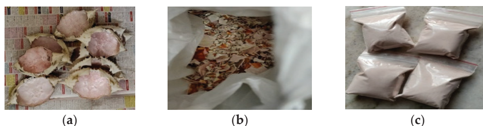
Figure 1. (a) Cleaned crab shells; (b) coarse particles of crab shells; (c) crab shell powder.
