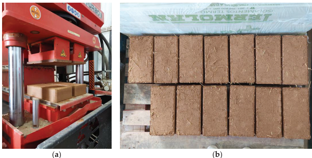
Figure 5. (a) Freshly manufactured blocks and (b) batch of blocks (mixture WS15) ready for curing.
