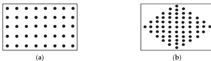
Figure 2. (a) Even distribution of porosity; (b) uneven distribution of porosity.
