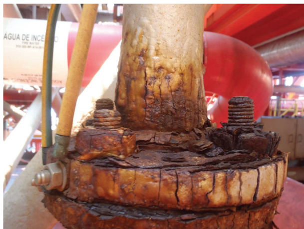
Figure 4. Degradation of an FPSO pipeline due to galvanic and differential aeration corrosion after five years of operation.
