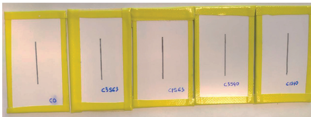
Figure A2. Coated samples before the FFC test. A 3 cm longitudinal scratch is introduced in the organic layer.
