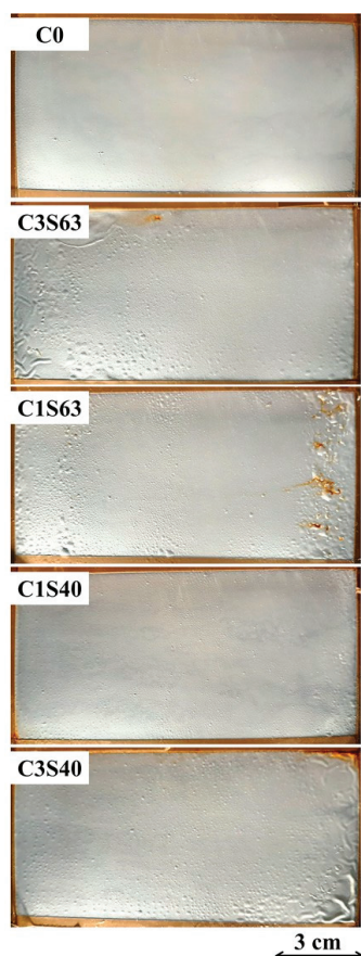
Figure 5. Coated samples after 1000 of NSST exposure.
