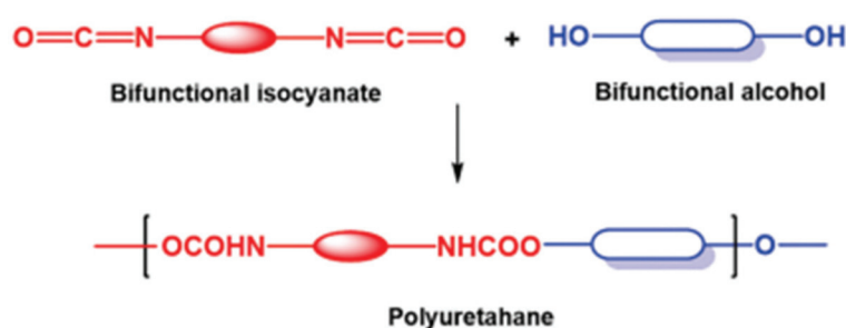
Figure 2. Addition reaction to synthesize polyurethane. Reprinted from [47].
