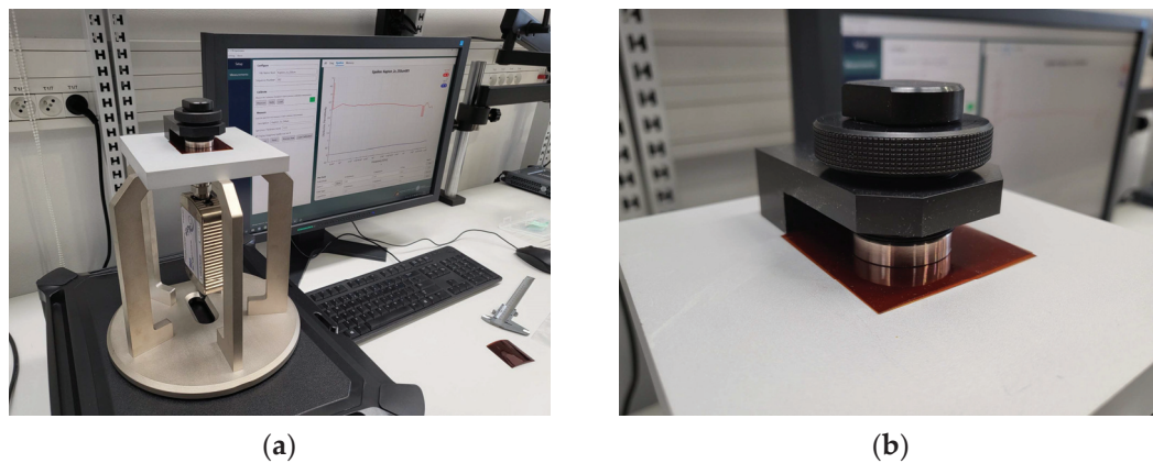
Figure 16. Laboratory research stand: (a) epsilon meter; (b) piece of Kapton under testing conditions.
