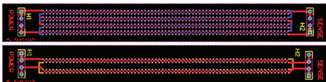
Figure 2. Design of samples, with the two-layer PCB above and the four-layer PCB below.
