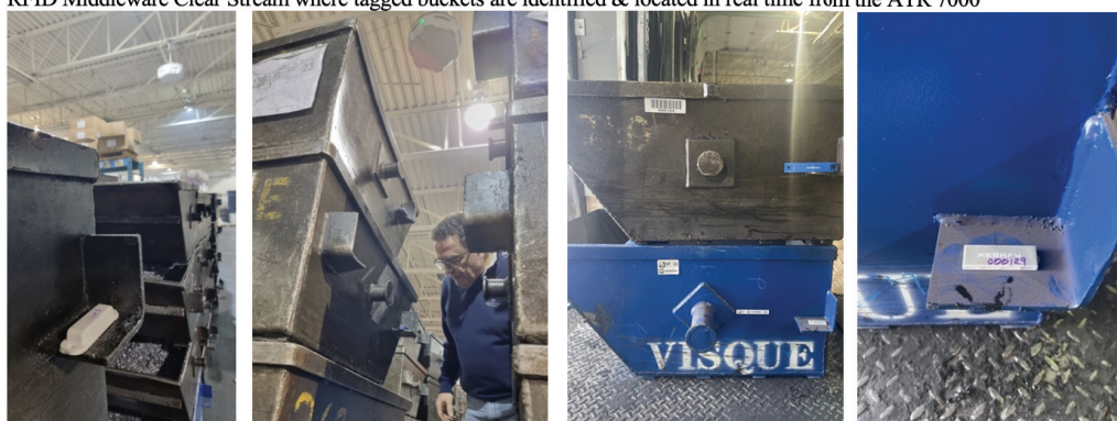
Slecting the “right” tags &amp; tag placement to identify the buckets (and maximise the chances to be detected)
