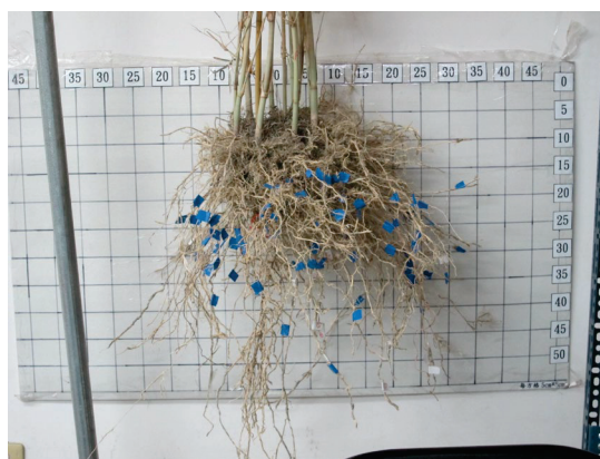
Figure 3. The Pachi bamboo root system at the test site (the numerals shown in the figures are in units of centimeters; the blue tag in the photo is used to facilitate the counting of roots with different diameters).
