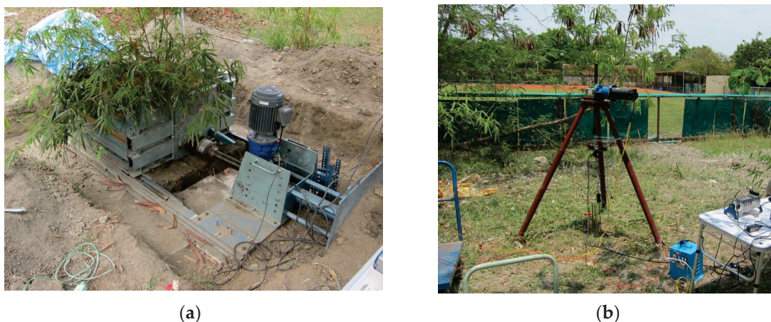
Figure 2. The apparatus of in situ mechanical tests. (a) In situ shear test; (b) in situ pullout test.
