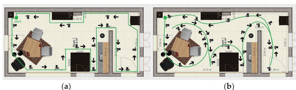
Figure 4. (a) Method 1: Following the contours of the whole environment, (b) Method 2: Circle around the main objects in the rooms in one path.
