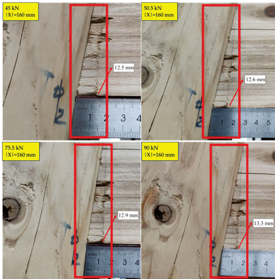
Figure 5. Pull-out lengths of tenons across four different load conditions.
