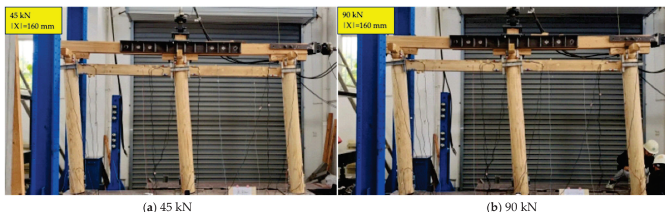
Figure 4. Rotational deformation of the column frame under varied vertical loads: a comparison of 45 kN and 90 kN load conditions.
