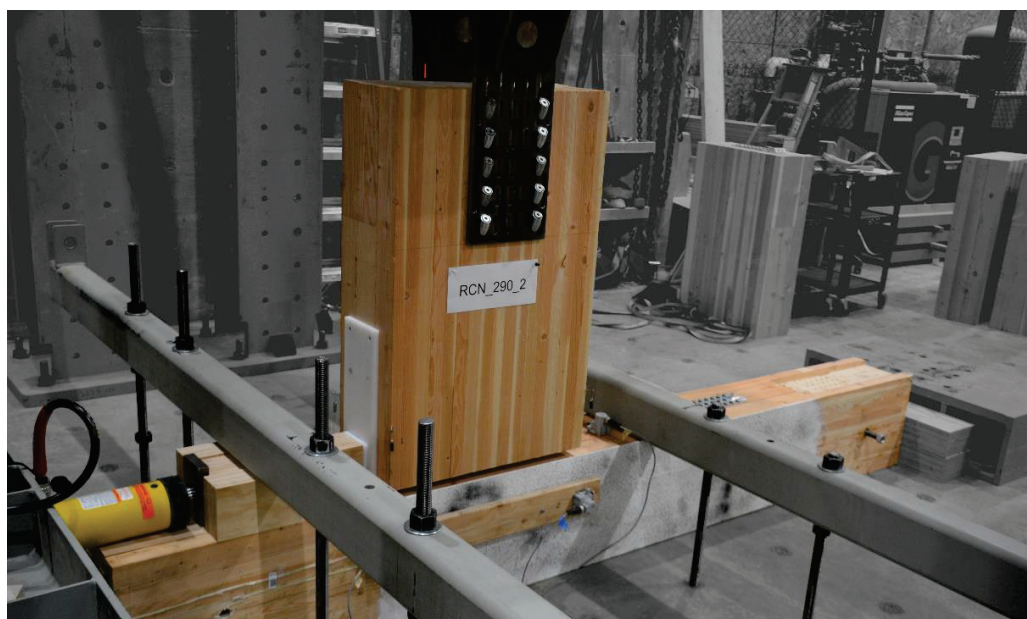
Figure 4. Biaxial loading test set-up.
