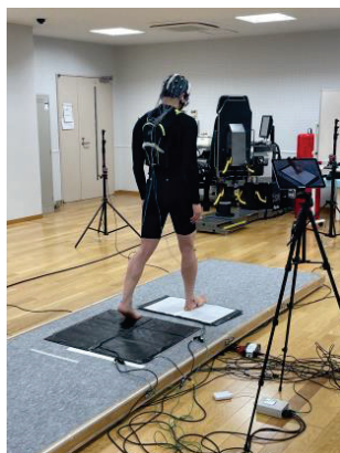
Figure 1. Experimental setup. The participant is wearing a 28-electrode EEG cap while standing on the pressure-sensitive mat system. The black mat in front of the participant is the initial position mat, and the white mat is the target position mat. Small markers were placed on the posterior and lateral sides of the calcaneus to precisely measure heel contact points. An iPad was used to record stepping movements. Participants performed 20 stepping trials, aiming to align their heels with the designated target point. EEG: electroencephalography.
