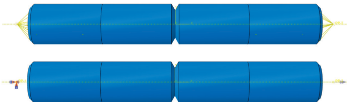
Figure 12. Notched specimen coupling relationships and loads.
