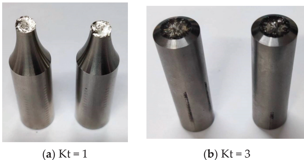
Figure 6. Fracture morphology of room-temperature specimens.
