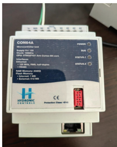
Figure 3. Programmable controller operating as smart thermostat.
