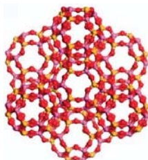
Figure 8. Schematic structure of Faujasite type zeolite. Reproduced from reference [77] under CC BY 4.0.
