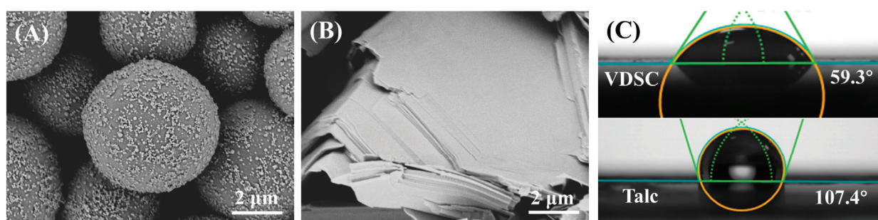
Figure 3. SEM images of (A) VDSC and (B) talc. (C) Contact angles of pure VDSC and talc to film-forming agent solution.
