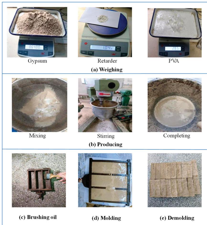
Figure 4. Manufacturing process of PVA gypsum blocks.
